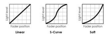
Figure 4. Dimming curves
