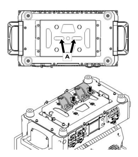
Figure 7. Rigging brackets directly mounted
