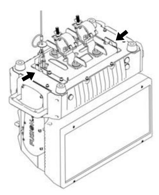
Figure 4. Safety cable attachment
