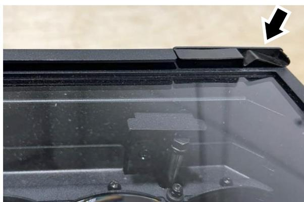
**Figure 7. Front cover retaining clip**
