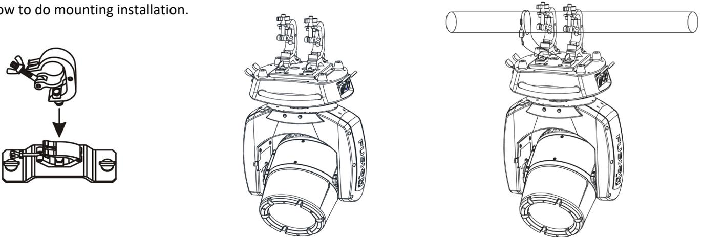
Step one: Installation the clamp onto the omega bracket;
