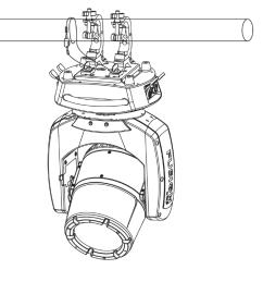
Step one: Installation the clamp onto the omega bracket;
