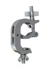
The trigger clamp is a clever combination of c-clamp and half coupler and is ideal for securing heavy devices. The trigger clamp is easy to hang and guarantees a certain level of drop safety, even when the clamp is still open, making it easy for someone working alone.
