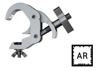
The Self locking Hook Clamp is a fast and simple way to attach devices to a truss. The special design with lateral screw prevents it from hooking itself to the devices or to the cross beam. The large wing nut makes it easy to lock the clamp in place.
