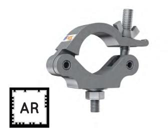
The half coupler is the standard in heavy duty clamps and can accommodate up to 1100 lbs tensile load. Due to its width, it offers substantially more load bearing surface, and is thus better secured.
